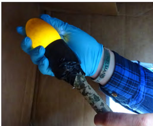
Figure 2. Egg candling using a modified Cree XPE High Power LED® as oviscope inside a cardboard box
