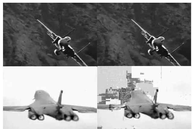
Fig. 10: Captured video stream on the transmitter (left side) and receiver (right side) for two cases. In the first case (upper figures) without packets lost and in the second case (lower figures) distortions appears on receiver caused by lost packets.
