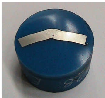
Figure 4: Polished and etched sample ready to be measured for hardness.
