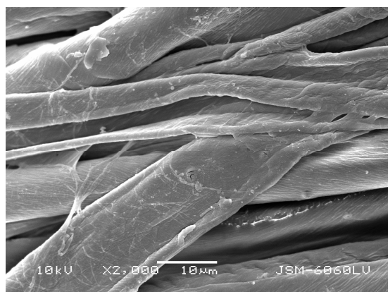
Figure 5. Surface of fibres coated with a layer of \text{ZnCl}_2 and alginate.
