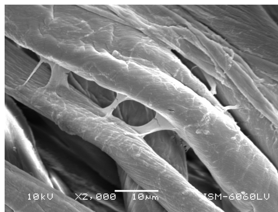
Figure 3. Film of ZnCl_2 and alginate on fibres and between them.
