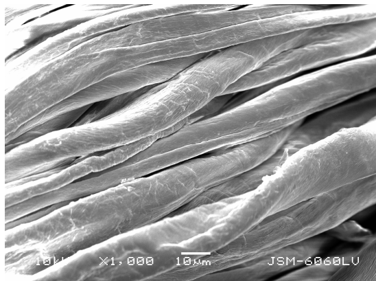
Figure 1. Cotton fibres impregnated with 3M ZnCl_2 .
