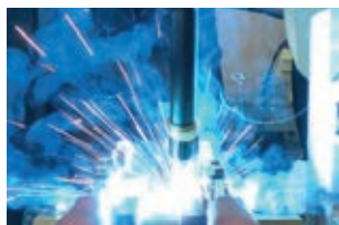
» Kontroliran prehod materiala - Controlled modified short arc
