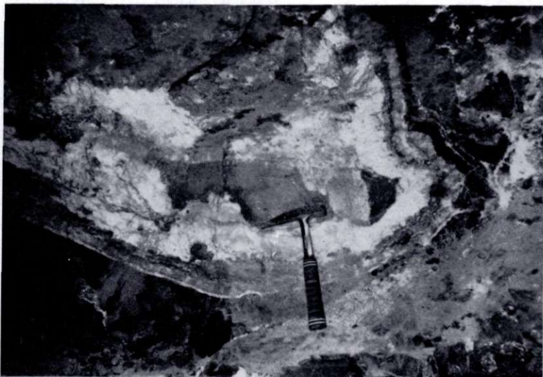
Fig. 3. S. Giovanni Mine. "Ricchi Ag" stope. Sardinia (Italy). Fragment of Cambrian carbonatic rock surrounded by prevalent calcite (white) and quartz-galena (grey to black).
