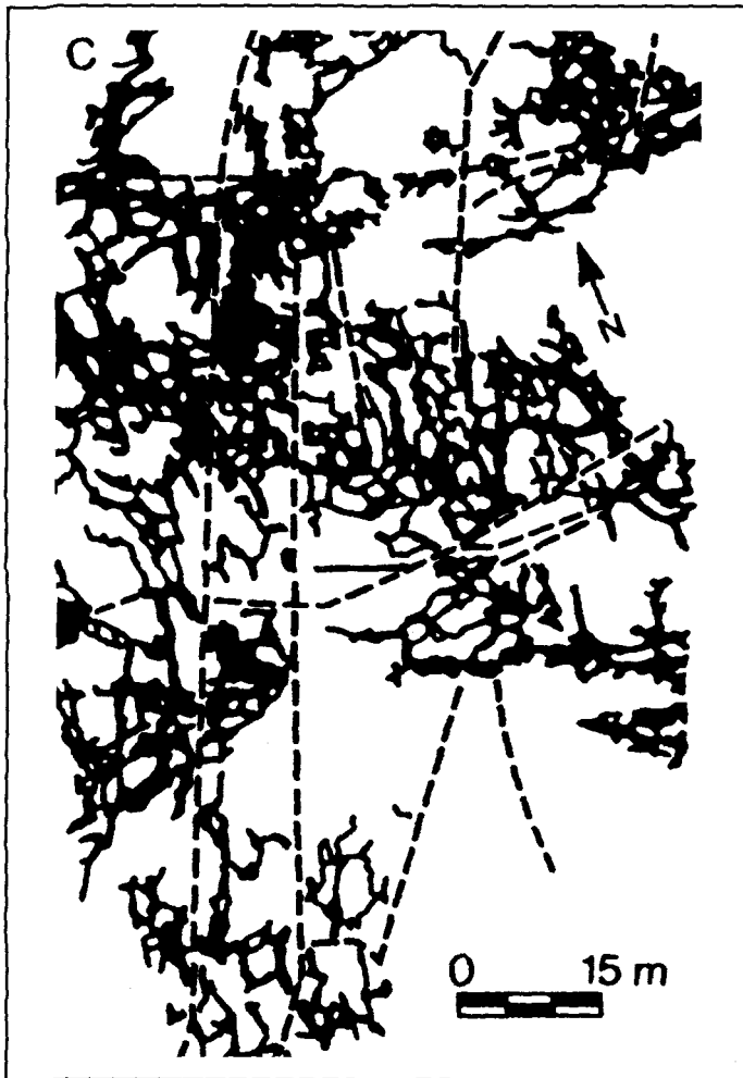
Fig. 7: Section of the Jefferson City Mine, Tennessee, where black is used to indicate galena deposits; it is evident how the mineralization has completely fossilised the 3-D maze karst system (from FORD & WILLIAMS, 1989, modified)
