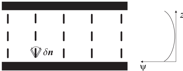
Figure 5.3 Homeotropic nematic cell with surface induced presmectic order \psi . The profile of positional order is shown schematically. We consider the Casimir force induced by the director fluctuations \delta\mathbf{n} .
