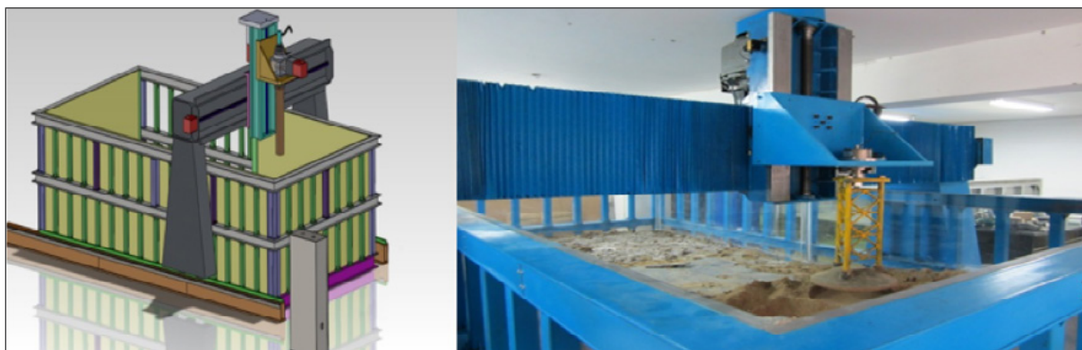
Figure 2. Pile-soil interaction experimental facility.
