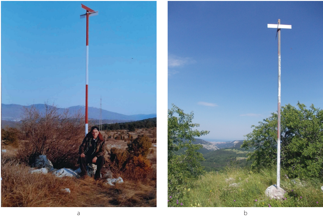
Figure 10: Metal target signals: a) at the installation time in 1996 – Soline above the village of Beka, 3 rd order, No. 87, C0, trigonometric district Sežana; at the foot of the metal signal sits Ivan Lojtk (photo: archive of I. Lojtk), b) today – Črna griža, 4 th order, No. 47, C0, trigonometric district Sežana (photo: R. Škafar, 2021).
