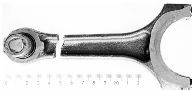
Figure 1: Connecting rod's fractured shank
