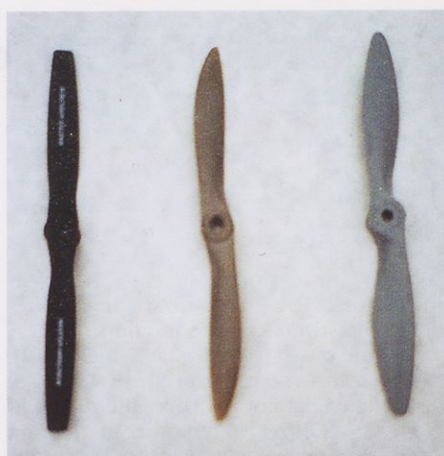
Slika 6. Testni propelerji: Master Aircsrew 9 x 4, APC 9 x 4 in Aviomodelli 9 x 4
