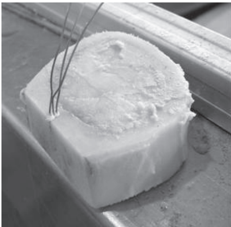
Fig. 2. Preparation of the hollow bone segments (specimens)
