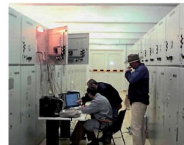
Figure 4: Electromagnetic compatibility testing inside a power substation
