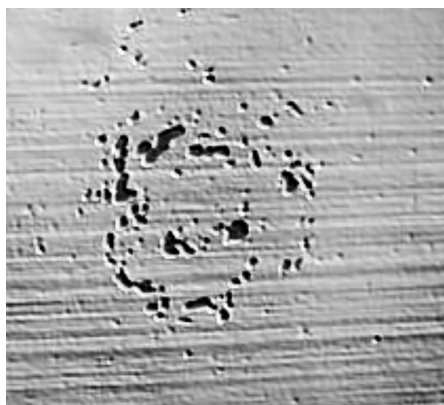
Figure 1: Cross-section at half ingot body height. Image of liquid penetrant test and detail of the axial part of the 8CrMoSiV steel ingot Slika 1: Prečni prerez pri polovici višine ingota. Posnetek preiskave s tekočim penetrantom in detajl aksialnega dela ingota iz jekla 8CrMoSiV
