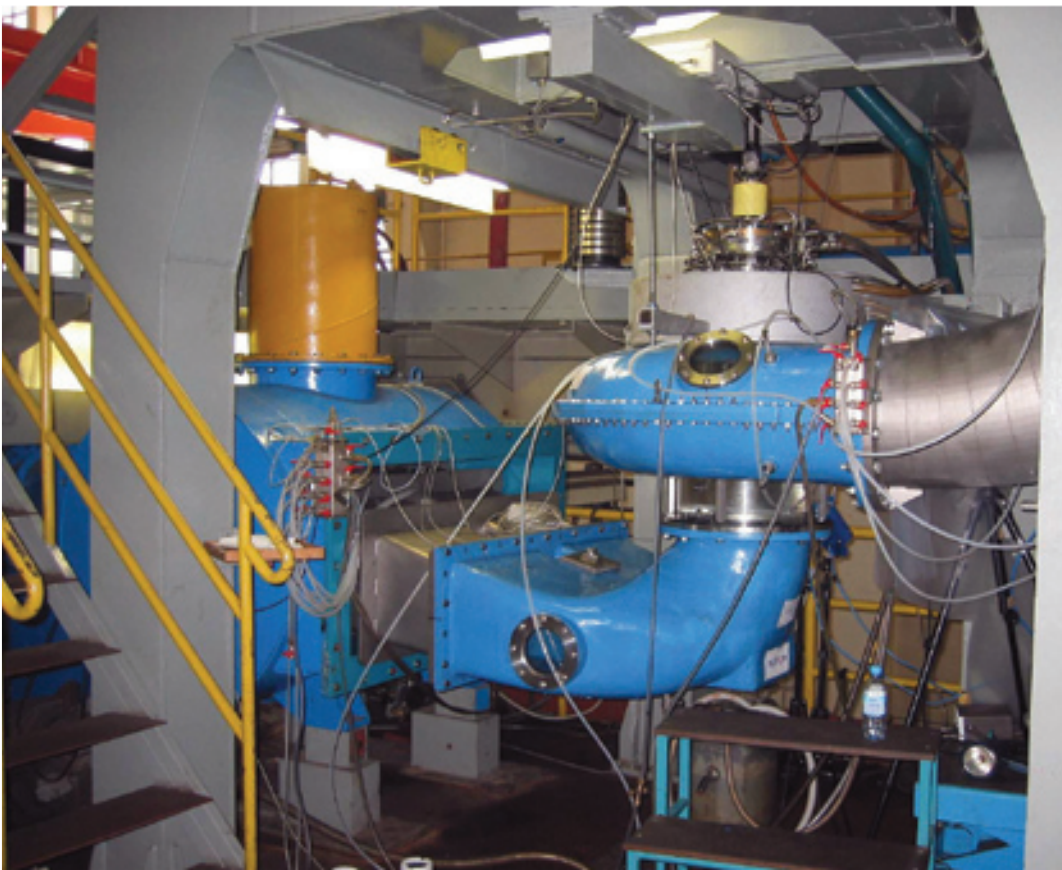
Francis turbine model on test rig
