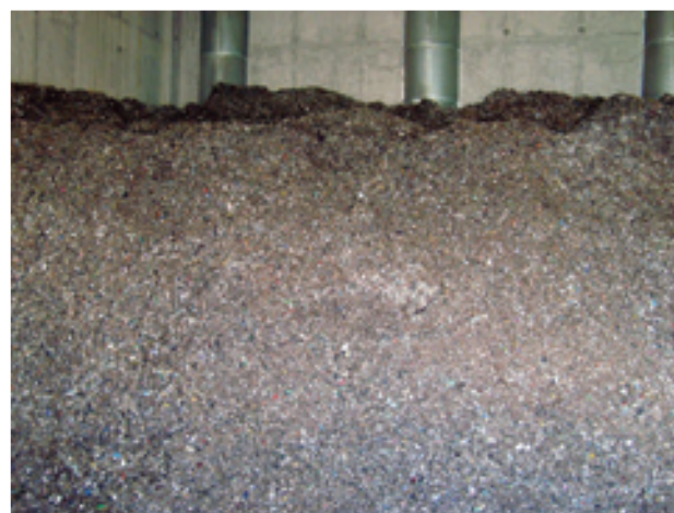
Fuel – Light fraction of waste, prepared for incineration, is almost free of the odour typical of most municipal waste.
