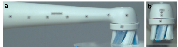
Fig. 3. Brush head with tracking markers in a) side- and b) front view
