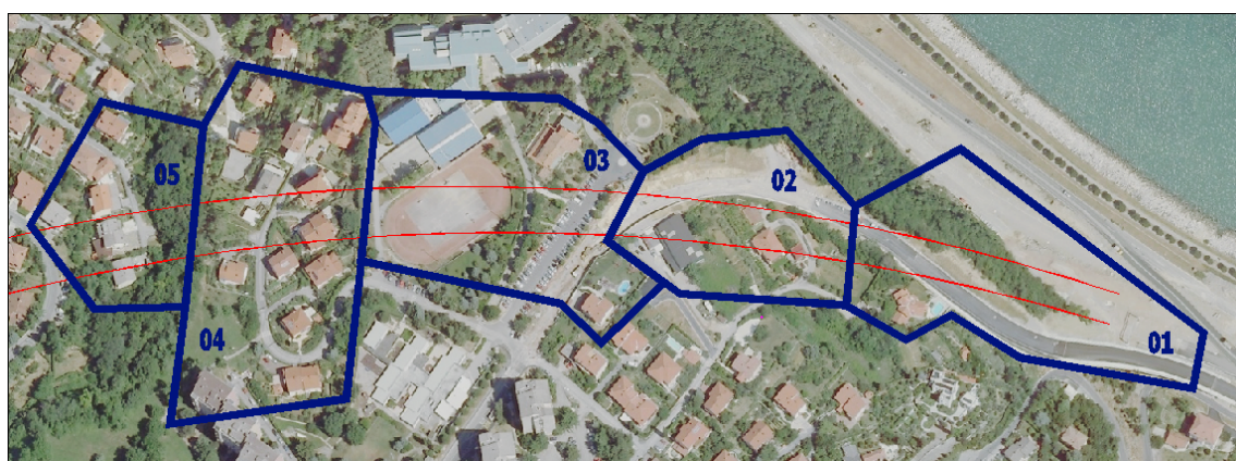
Figure 40: Sectors selected for monitoring excavation effects. So-far only Sector 1 was excavated, limiting the deformation inspection of the thesis to this particular area. The red lines represent the two tunnel axes.
