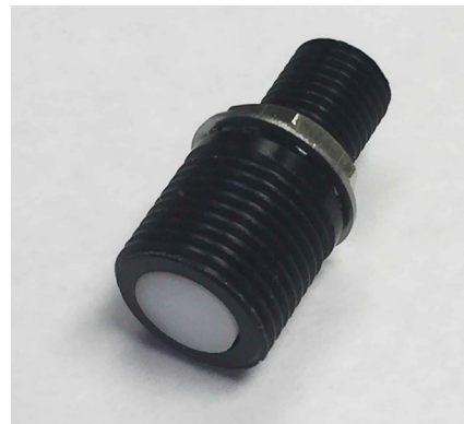
Slika 31: Kosinusni receptor s 180° vidnim kotom zajemanja. Figure 31: Cosine receptor with 180° field of view.
