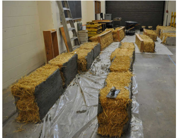
Slika 3: Priprava merjencev – nanos ometa na bale slame. Figure 3: Specimen preparation – straw bale plastering.
