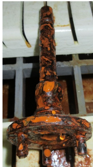
Fig. 3 Specimen (steel planetary axles) positions in the NSS chamber equipped with air flow operating aqueous salt spray nozzles
