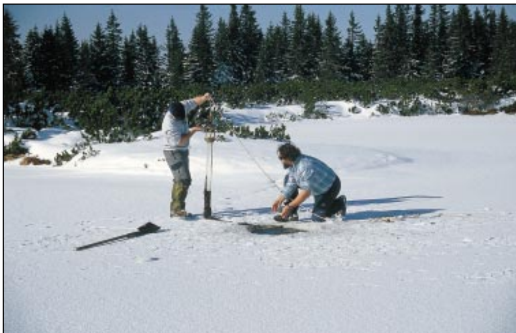
Figure 8: Collecting a sample of the sediment with modified Kajak sediment sampler on frozen Lovrenška jezera (lakes, October 1998, photography Anton Brancelj).
