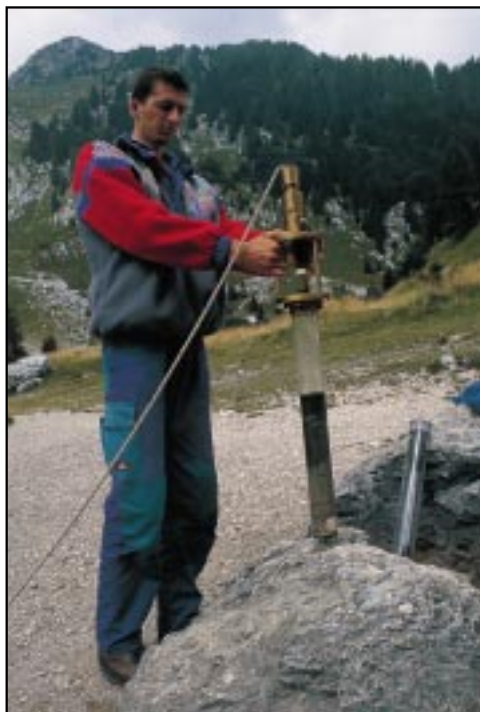
Figure 9: Modified Kajak sediment sampler with a sediment core (Lake Krnsko jezero, Slovenia; September 1998).
