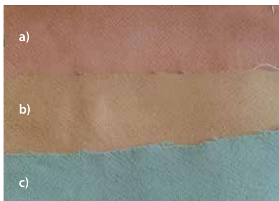
Figure 3: Wool dyed using MDF sawdust with different mordants: a) ferric sulphate, b) potassium dichromate and c) copper sulphate
