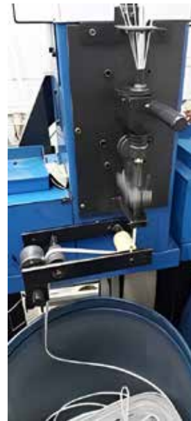
Figure 2: Cord knitting machine – internal cylinder diameter (cord diameter) = 6 mm
