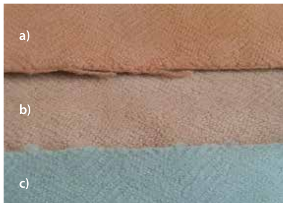
Figure 2: Wool dyed using eucalyptus sawdust with different mordants: a) ferric sulphate, b) potassium dichromate and c) copper sulphate
