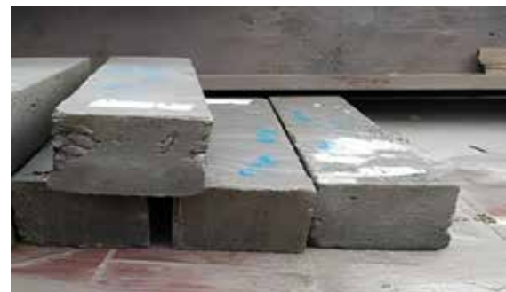
Figure 6: Reinforced concrete beams with PP prepared bars
