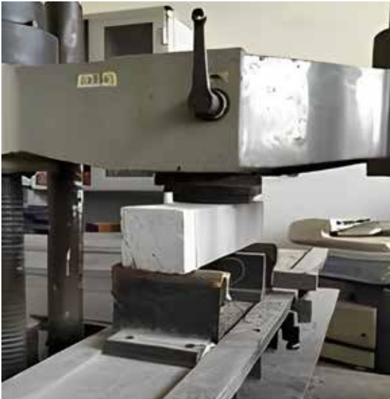
Figure 7: Flexure point load test of reinforced beam with the PP cord-knitted bars
