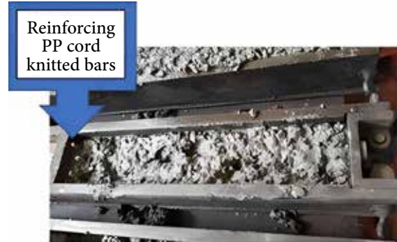
Figure 5: Pouring reinforced beams with PP prepared bars
