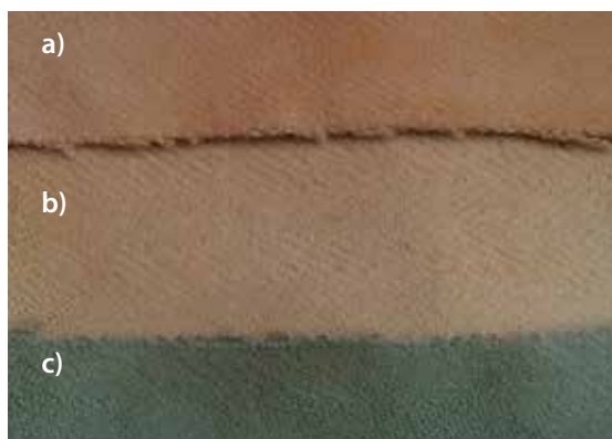
Figure 4: Wool dyed using wonza sawdust with different mordants: a) ferric sulphate, b) potassium dichromate and c) copper sulphate
