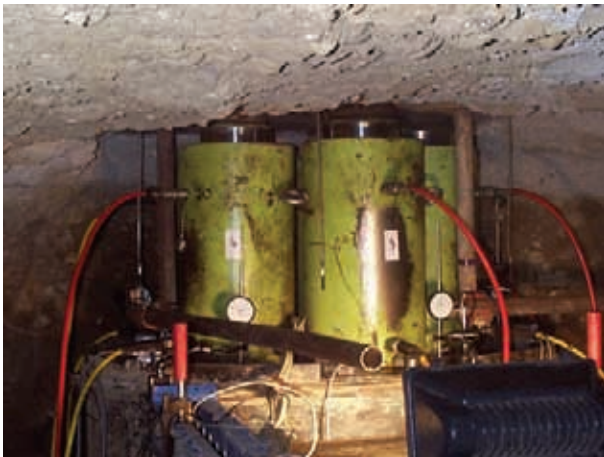
Figure 2. Hydraulic jacks and measurement equipment in the beginning of loading test.
