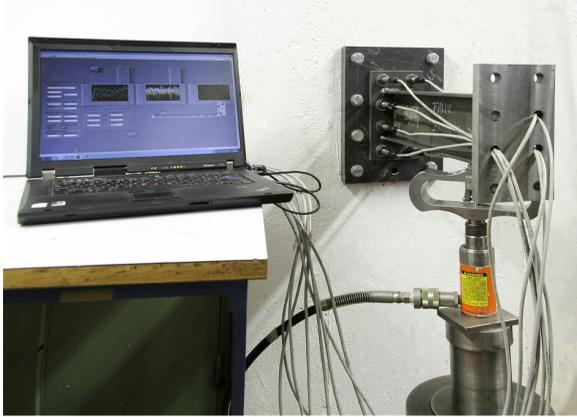
Fig. 10. Discussed cantilever beam with measurement and loading equipment
