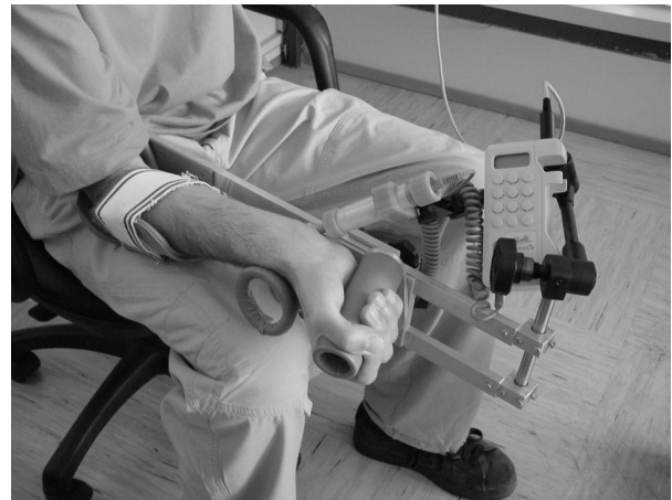
Figure 1 Custom designed arm attached Doppler velocity measurement probe holder
