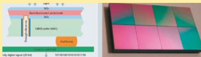
Figure 3: Schematic drawing shows the configuration of the new Stellar Detector. The light from the UFC scintillator reaches the back-illuminated photodiode on top of the CMOS wafer that contains the ADC. The digital signal is then produced on the other side of the wafer (Fig. 3A). A picture of the compact Stellar Detector array with the ADC positioned entirely underneath the photodiode array (Fig. 3B).
