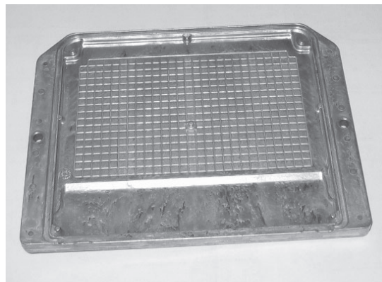
Fig. 1. Electronic component support made by aluminium high pressure die-casting
