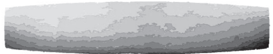
Fig. 11. Visualization of D_k on casting E_4. (light: +0.04 mm above R_k , dark: -0.04 mm below R_k )
