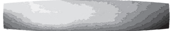
Fig. 9. Visualization of D 1 on casting E_2. (light: +0.7 mm above R k , dark: -0.7 mm below R k )
