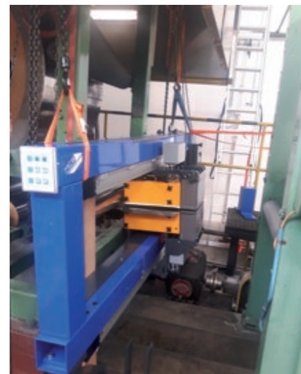
Merilni okvir na koncu papirnega stroja Measuring frame at the end of the paper machine
