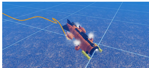
Figure 6: The ROV being rendered in Godot, visualizing a recorded dive and drawing a trail behind the vessel.
