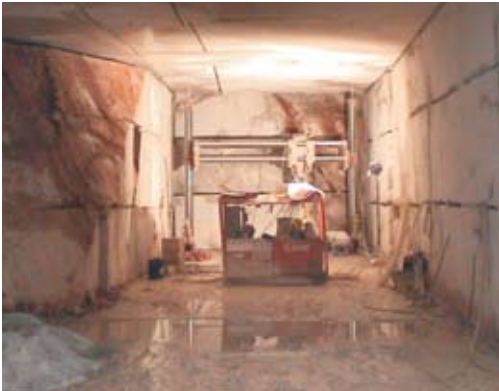
Figure 6. Stope face with underground mining of natural stone
