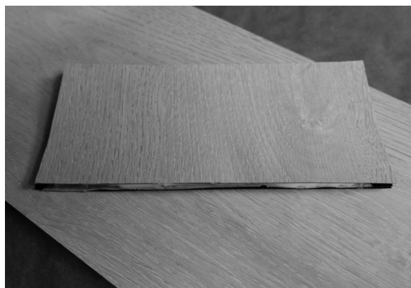
Fig. 14. Sample of pressed layers of WDSM flooring
