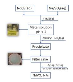
Fig. 1. A schematic representation of the synthetic procedure to obtain  $\rm NdVO_4$  nanoparticles.
