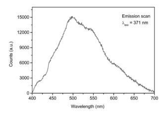
**Fig. 8.** The emission spectrum of NdVO<sub>4</sub> nanoneedles, measured at room temperature.
