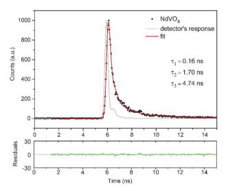
**Fig. 9.** Photoluminescence lifetime measured on the NdVO<sub>4</sub> nanoneedles,  $\lambda_{em} = 524$  nm. The black dots represent the time-domain intensity decay. The red line is the fitting curve, while the grey line is the response of the detector. The green line below represents the difference between the fitted curve and the measured data. The goodness of fit,  $\chi^2$ , is 1.418.
