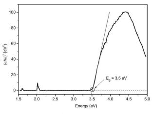
Fig. 7. Optical band gap of NdVO<sub>4</sub> nanoparticles.
