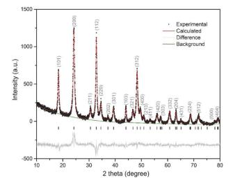
**Fig. 2.** X-ray powder diffraction pattern of the  $NdVO_4$  nanopowder. The black full circles represent raw data and, red solid line is the Rietveld fit, the black vertical bars are the Bragg reflections, while the grey line shown below is the difference between observed and calculated intensity.
