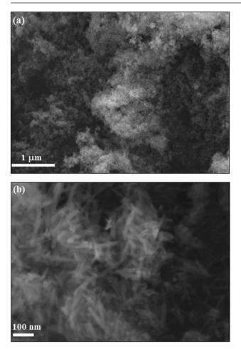
**Fig. 3.** SEM images of the NdVO<sub>4</sub> nanopowders. (a) Low magnification, (b) High magnification.
