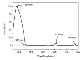
**Fig. 6.** The UV-Vis diffuse reflectance spectrum of the NdVO<sub>4</sub> nanopowder prepared in this study.
