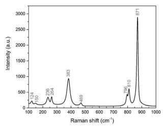
Fig. 5. Raman spectrum of the  $\rm NdVO_4$  nanoparticles prepared in this study.
