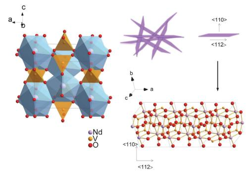
Fig. 4. (a) Crystal structure of NdVO<sub>4</sub>; (b) Schematic representation of the as-grown NdVO<sub>4</sub> nanoneedles; (c) Ball-and-stick model showing a tetragonal NdVO<sub>4</sub> nanoneedle grown along <112>.
