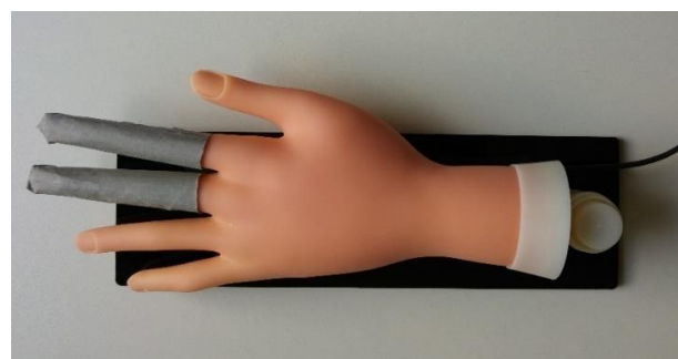
Figure 6. EDA simulator shaped as a human hand with active electrodes on the index and middle finger [2].
