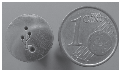
Sl. 4. Elektroda za PPME, izdelana z VC Fig. 4. MEDM electrode machined with WJ technology
