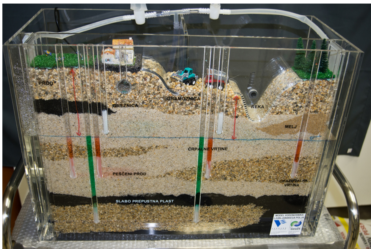
Sl. 1. Gladina vode v modelu vodonosnika (modra črta) in globina do podzemne vode (rdeča puščica) Fig. 1. The groundwater level in the aquifer (blue line) and the depth to the groundwater (red arrow)
