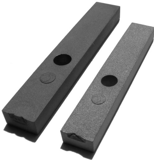
**Figure 7:** Green and sintered specimens used for the analyses
