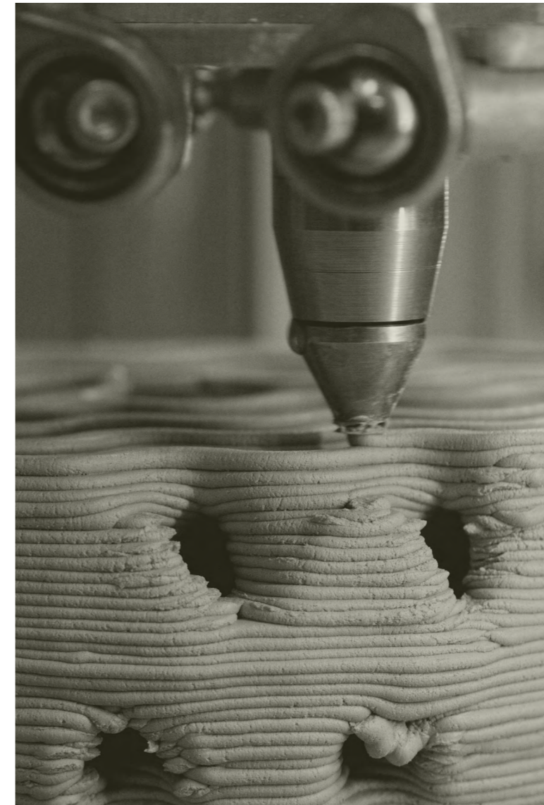
Dodola I : Sustainable water filtration product produced using 3D printing technology, containing principles of gyroidal structure and Archimedean screw
