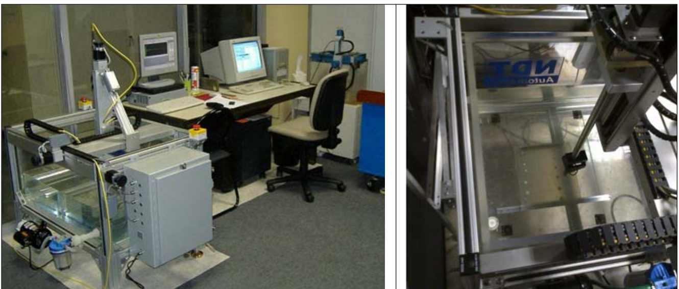
Figure 4. ULTRAPAC system (on the left); GRPC plate in the immersion tank (on the right)
