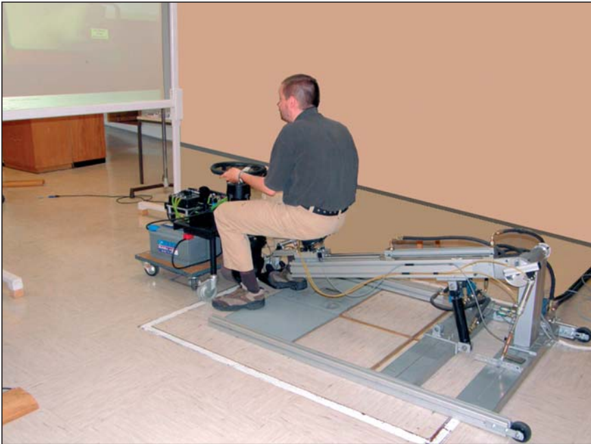
Figure 7. Experimental evaluation of robot environment for combat vehicle driving simulation
