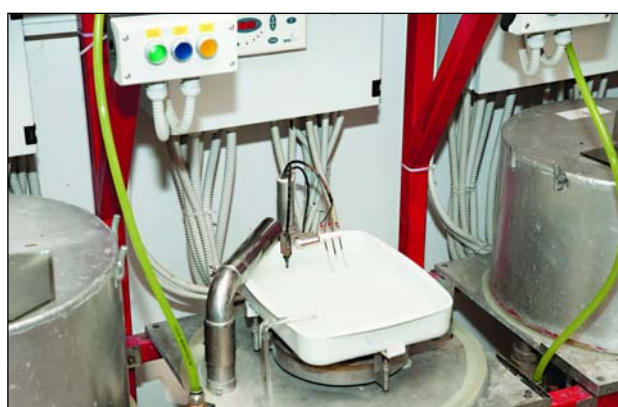
Figure 5. Photograph of the interior of the sample-evaporation chamber.
