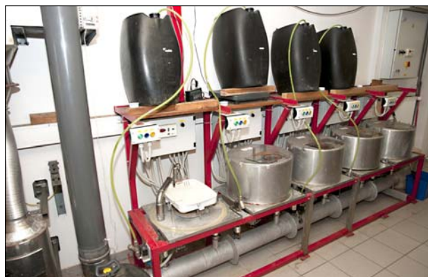
Figure 4. Photograph of the evaporation apparatus with the first chamber cover removed.
