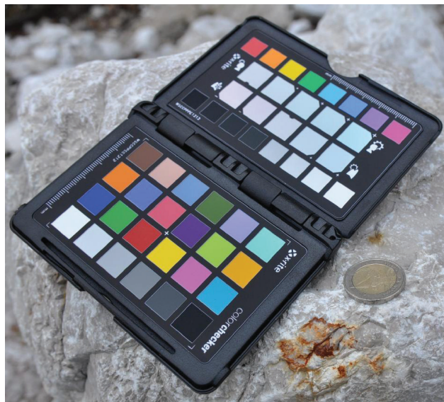
Fig. 3. X-Rite ColorChecker Passport colour calibration chart that is used by our application.
