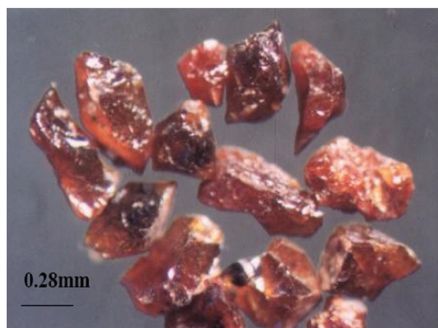
Fig. 2. Samarskite-Y crystals exhibiting massive granular shape with reddish brown colour, Binocular microscope
