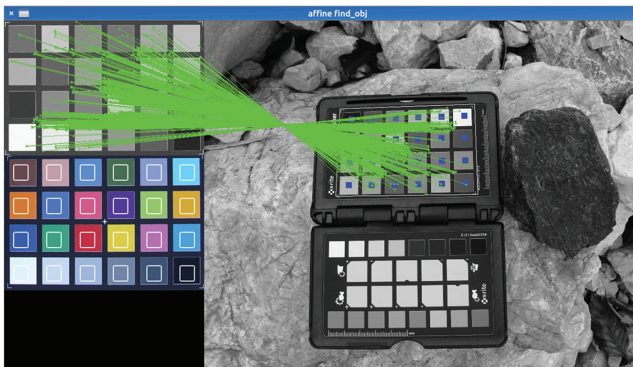
Fig. 4. Visualization of ASIFT on a photograph of X-Rite ColorChecker Passport (right hand side) and reference X-Rite ColorChecker Passport colour patch image (upper left hand side).
