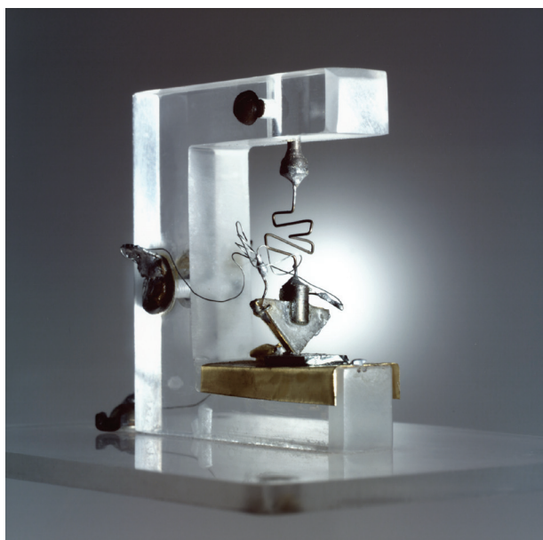
Figure 3: First transistor. Reprinted from [8]. Copyright 2020 Nokia.
