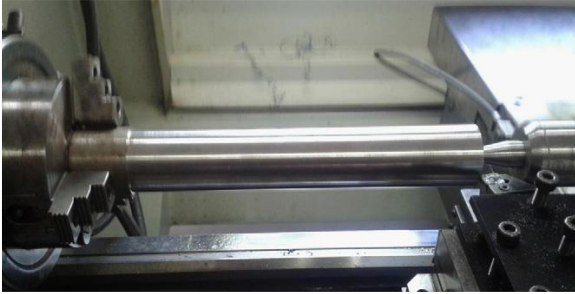
Fig. 3. AISI 12L14 free machining steel turning process
