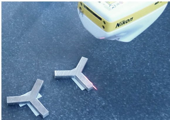
Fig. 6. Part measurement with a non-contact laser scanner
