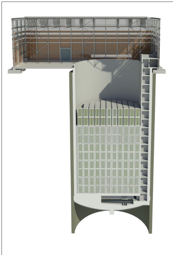
Figure 17: The LILW disposal silo and the hall above the silo, as shown in the design for the construction permit
