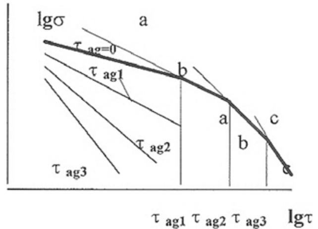
**Figure 3:** Schematic representation of the method of extrapolation. Vertical lines represent the stage of softening of the material during the aging process (Lines bb and  $\tau_{ag1}$ , cc and  $\tau_{ag2}$ , dd and  $\tau_{ag3}$  are parallel)
