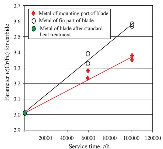
**Figure 1:** Dependence of the parameter  $w(\text{Cr}/\text{Fe})$  of the metal from different parts of low-pressure turbine blades on the service time
