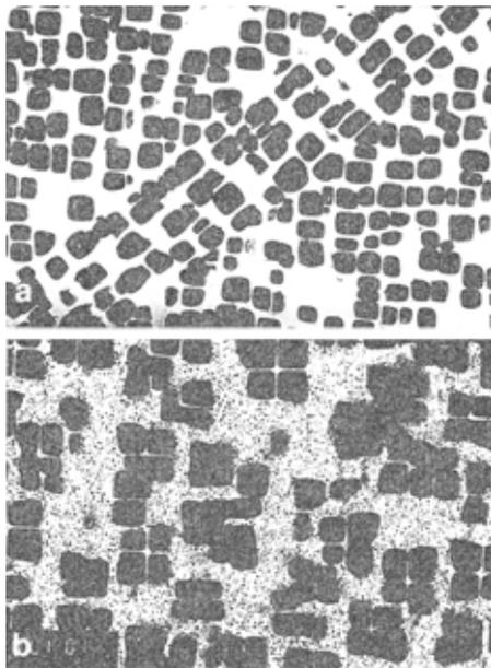
**Figure 6:** Electronic photos of microscopic structure of the blade mounting part (a) and front fin edge (b) made of the alloy EI929VD (after 31043 h of service)
