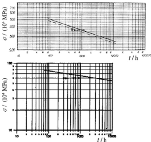
**Figure 8:** Long-term service influence on long-term strength of the alloys IN738 (a) and CNK-7 (b) – specification: experimental data for blade metal after operating time of 30,000 h
