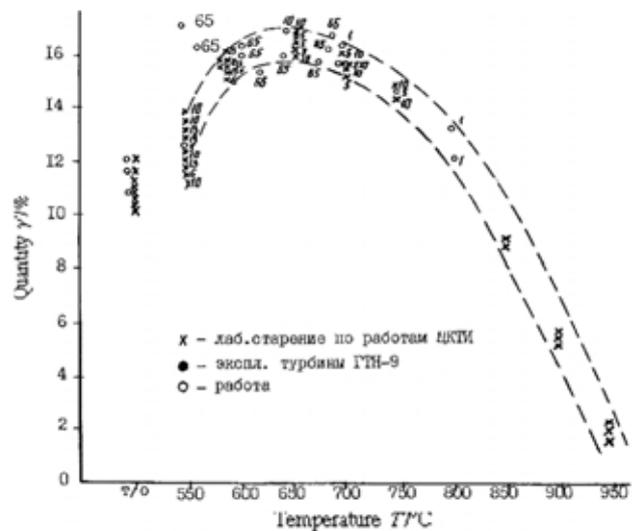
**Figure 4:** Influence of temperature on quantity of  $\gamma'$  – phase in the alloy EI893 after long-term blade service
