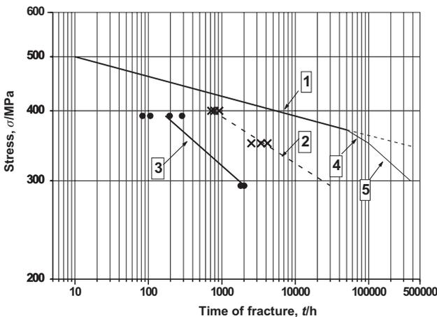
**Figure 2:** The long-term strength of blades made of steel EP428 under 500 °C
