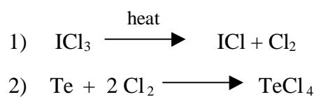
It is clear that at 250 °C, first some  $\text{ICl}_3$  dissociate to chlorine and iodine chlroride. Then tellurium reacts with fresh chlorine and forms yellow-green crystalline compound  $\text{TeCl}_4$ , which are separated from the vapour phase in the cold side of the ampoule.
