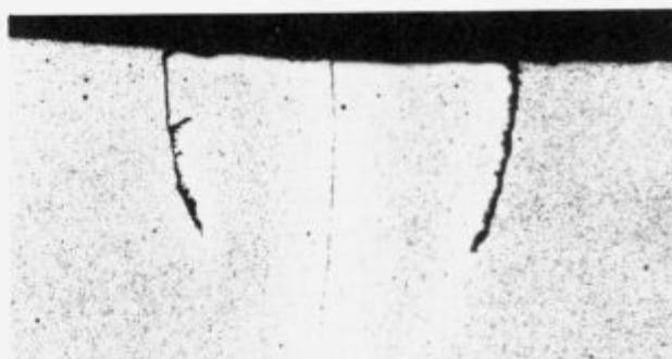
Slika 8. Obe vrsti napak: 1) v zvaru in 2) na robu toplotne cone. Povečava 100×. Figure 8. Two types of defects: 1) weld defect 2) edge from heat affected zone. Magn. 100×.
