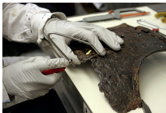
Figure 9: Careful removal of a small sample from a late medieval breastplate. (Photo: T. Lazar)
